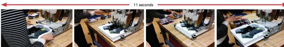
4) Operator actuates APU to start automation cycle
